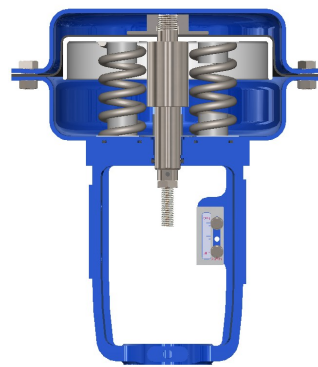
Figure 3. Cross Sectional Drawing Diaphragm Actuator (Reverse Acting)
